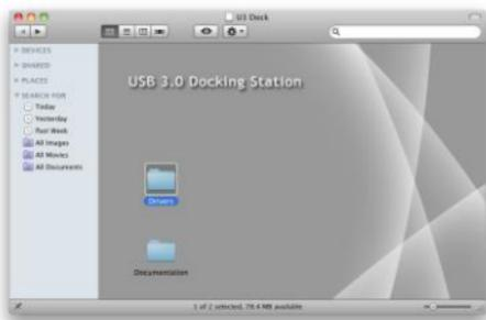
3. Select “**DisplayLink Software Installer**” to begin installing the DisplayLink Driver on your Mac.
